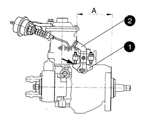
Insert wire rope through LFG basic lever.
